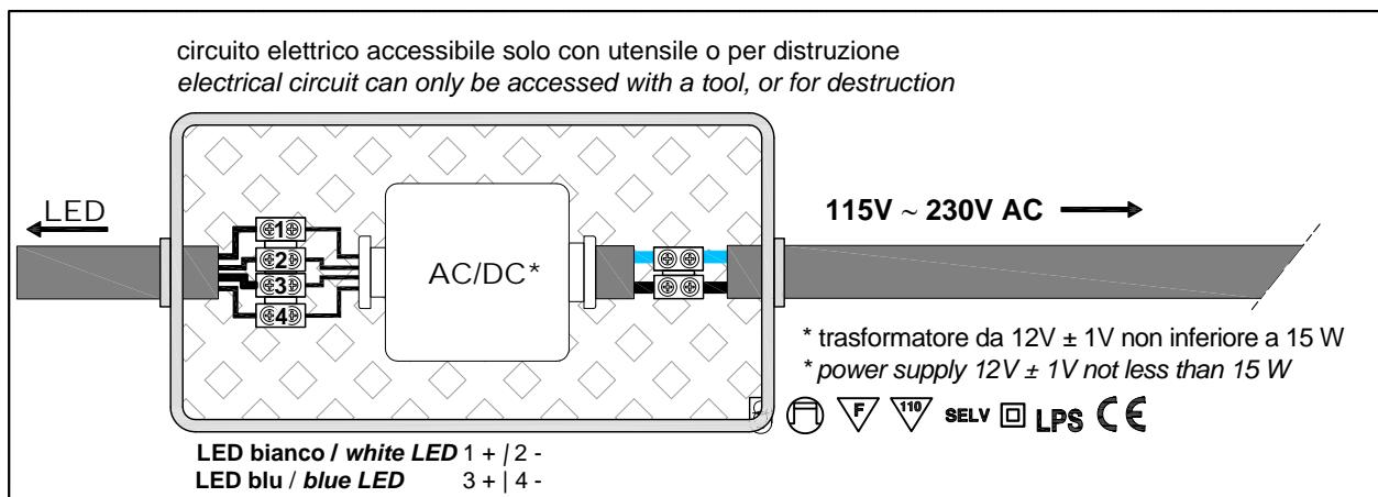
**CALICE** - Schema d'installazione / Installation layout
